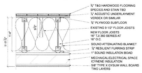
The minimum requried insualtion between floors is R-19 and we must also provide an uninteruped 1 hour fire sepeartion between the cellar level and 1<sup>st</sup> floor. The above floor makeup provides this as well as provideding an electrical/mechanical area that allows for the continuos 1 hr fire rating to be maintined.
